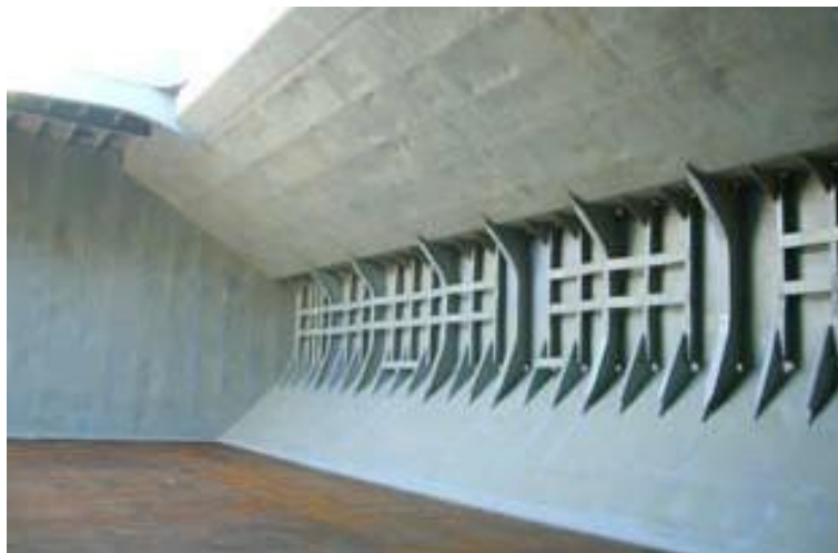
Hold of a bulk carrier that is grain clean and ready to load
