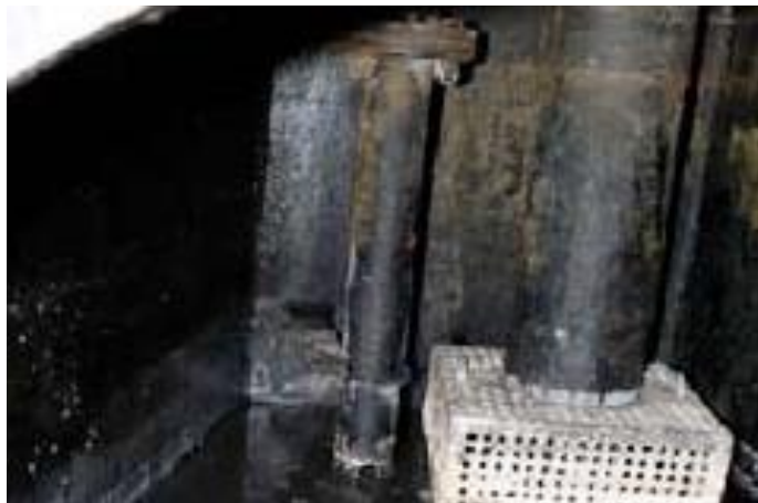
Check that bilge wells are clean and dry, and that strainers and strum boxes are cleaned
