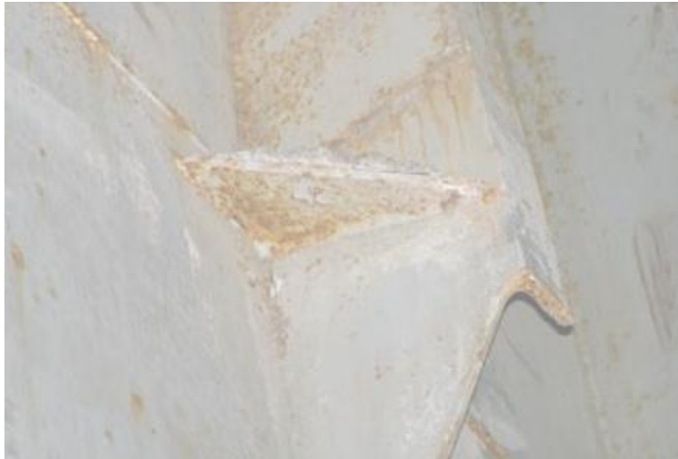
Residue of previous cargo will result in the hold failing the inspection to load grain
