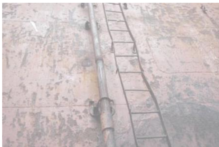
Flaking paintwork under the hatch coaming can result in a hold failing the grain survey
