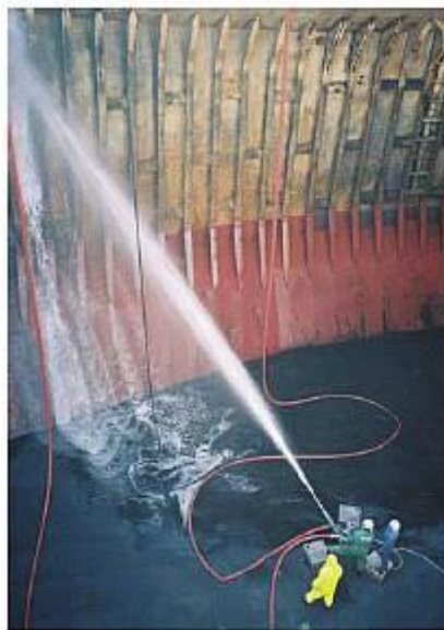
Typical hold cleaning equipment: crew operating a Toby gun and a Toby gun from Stromme.
